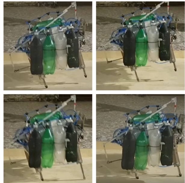
Fig. 2 Final trajectory of pneumatic quadruped robot
